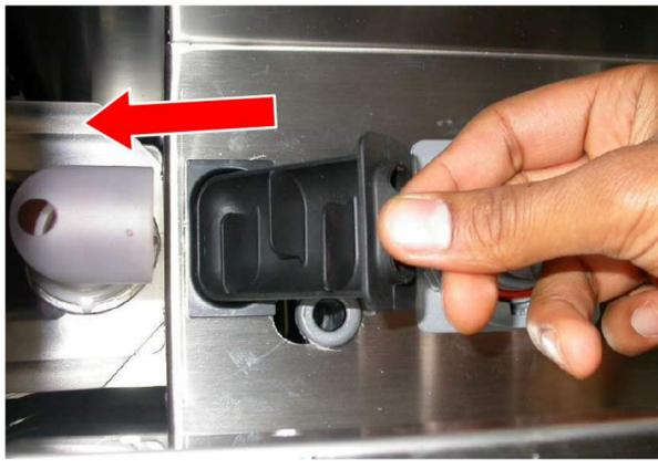
7 ▶ Turn the flange clockwise to reinsert the mixer
