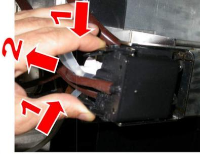
**3** ▶ Remove the milk frother from the coffee outlet and disconnect Silicone tubes No. -3- and -4-.
