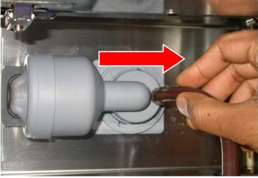
3 ▶ Turn the flange 1 anticlockwise, then remove the mixer 2
