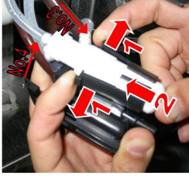
**4** ▶ Disassemble the milk frother in all its parts (first by turning and then by pulling as shown in the picture) and wash it either by hand or in a dishwasher. Make sure that all the holes are free from milk residues and also to use provided tools to clean the holes. Check also that the O-rings are in good condition
